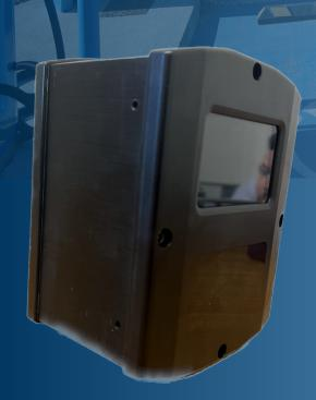
The all new Puma Bay Monitor Camera E has an aluminium extruded IP65 rated housing, integrated intelligent IR lights and processor making it a complete stand alone unit. The camera is fitted with a motorised Zoom/Focus lens controllable via the camera app enabling the user to set the perfect viewing area for a single bay. The camera utilises Suilvision core ANPR platform providing excellent plate reads 24/7.
